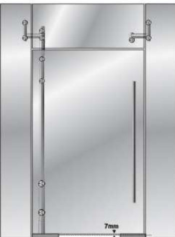
● JU800C-4 连体轴 Pivot pole with single point fixings and pivot bearing for intermediate tube 可提供各类型地弹簧接头 Can offer kinds of floor spring connections
