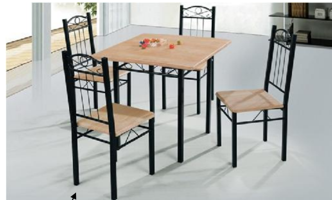
A088# Table , B086# chair , oak color , table 80x80cm for 1+4 steel frame , powder coated, mould pressed board, chair leg 25 x 25mm square tube (0.8mm thick) table leg 30mmx 30mm square tube
