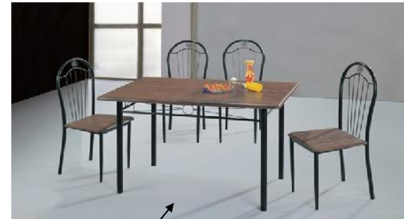
A083# table , B18# chair walnut color table 120x70cm , steel frame , powder coated, mould pressed board, chair leg 25mm diameter round tube (0.8mm thick) table leg 38mm diameter round
