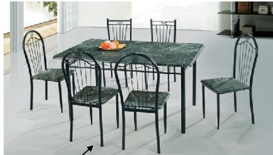
A084# table , B18# chair(round) green marble color table 120x70cm , steel frame , powder coated, mould pressed board, chair leg 25mm diameter round tube (0.8mm thick) table leg 38mm diameter round
