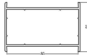
80Frame Connecting Profile (40) 80PG(40) 0.83kg/m
